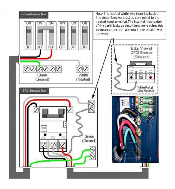
**Figure 3 – Cable schematics**Consult the caliber chart page 11
