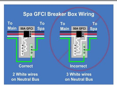
Figure 2 - GFCI Wiring
