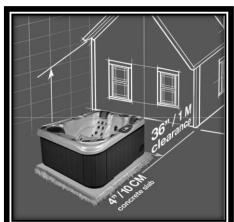
Figure 1 - Space Required (Clearance) and Support
