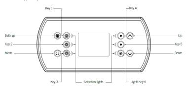
\* Functions for keys 1 to 5 will depend on your system's low level configuration.
