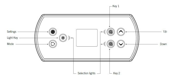
\*Functions for keys 1 and 2 will depend on your system's low level configuration.
