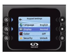
You can lock the keypad by selecting one of 3 security levels: Unlock, Partial or Full. The Partial level locks the set point adjustment and many options in the settings menu. The Full level locks all keypad functions. To unlock the keypad (either Partial or Full), press and hold the top right key for 5 seconds.
